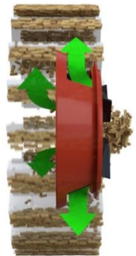
Even material distribution over the complete knife ring width
